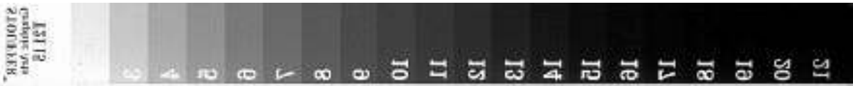
Figure adn3: A 21-step is scanned with a 12-bit scanner, with all features such as noise reduction and sharpening turned off, and the exposure adjustment set full range, and at 1200 ppi, full color with zero saturation.
