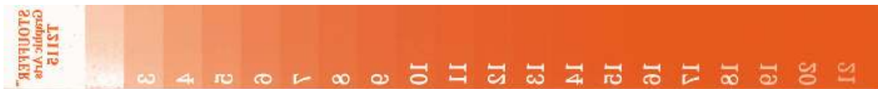
Figure 15b: 21-step after setting step 2 to the values of the Maximum Black Threshold.
