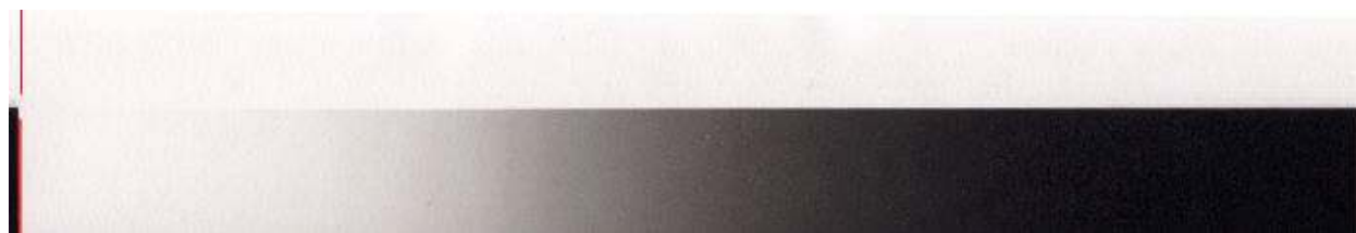
Figure 9: Using Pt/Pd print of the gradient to determine Maximum White (red indicator) for adjusting maximum deposition of printer inks. This example used the equipment settings described above.
